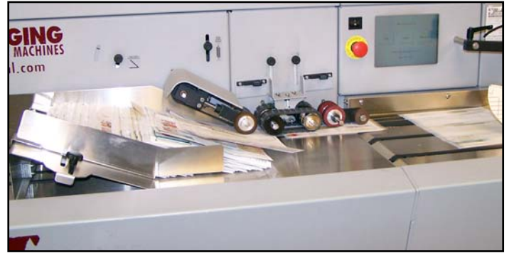
Documents and checks are a blur as they speed through the IBML ImageTrac III scanner transport
