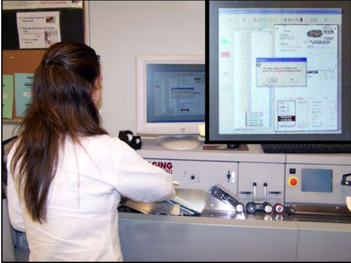
Inset: Quick Modules screen with scanned batches on the left, the full image on the right and a pop-up window providing an alert for the scanner operator
