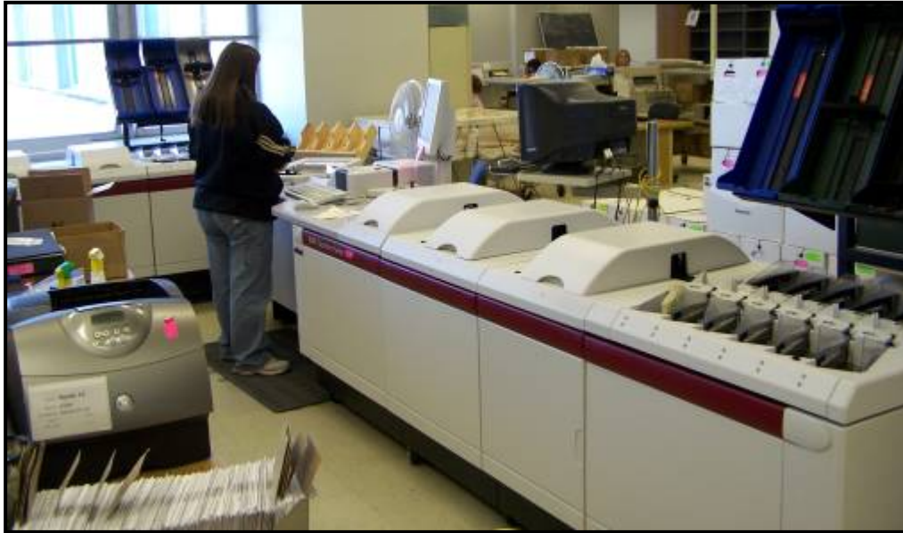
Chantel Lakey loads one of KDOR's Unisys NDP Quantum 300 Series payment processors with checks and voucher forms for tax payment processing.
