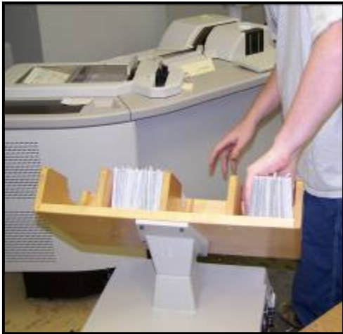
Vouchers and checks are evened up for processing in a vibrating form jogger.
